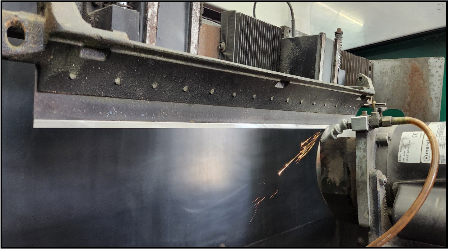
A photo of a bedknife being sharpened. The set up of a bedknife is equally important as the reel. Greens are mown at a height of roughly 0.100". The slightest imperfection makes a big difference.
