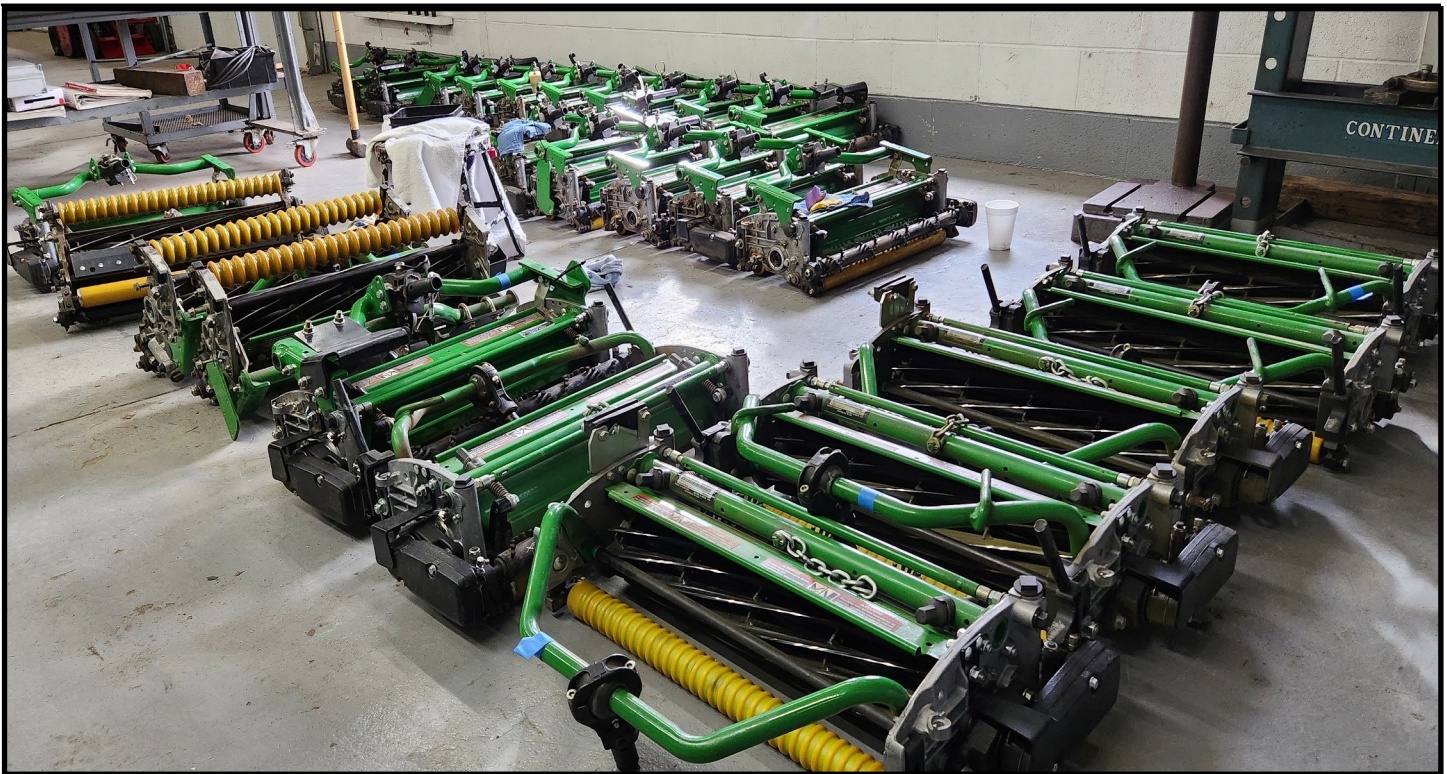
Fairway reels prepared for the grinder. There are 5 reels on each fairway mower, 3 reels on riding green and tee mowers and 1 reel on a walk mower. In total we have 59 reels for the machines used on greens, tees, and fairways.
